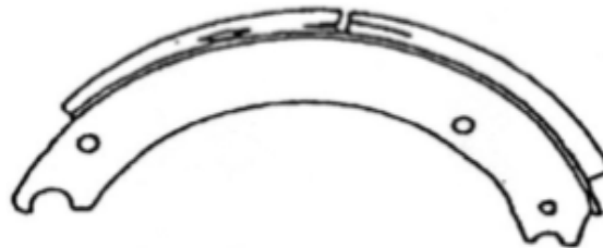
Out-of-Service Cracks or voids that exceed 1/16" in width. Cracks that exceed 1-1/2" in length.
